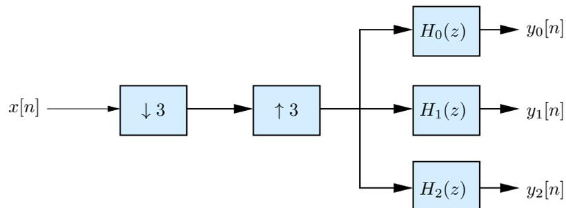
in which  $H_0(z)$ ,  $H_1(z)$  and  $H_2(z)$  are a lowpass, bandpass, and highpass filter, respectively, as follows:
