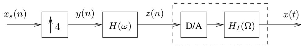
Figure 5: Block diagram of the oversampled D/A convertor.
