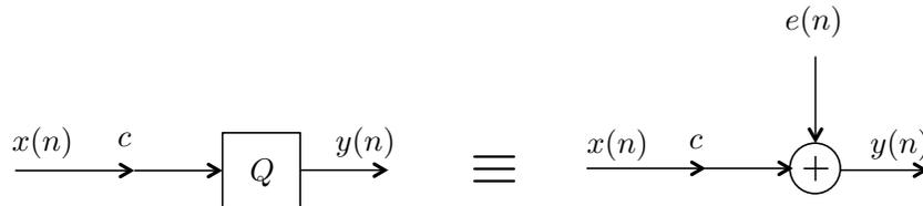
Figure 3: Additive noise model for quantisation noise.
