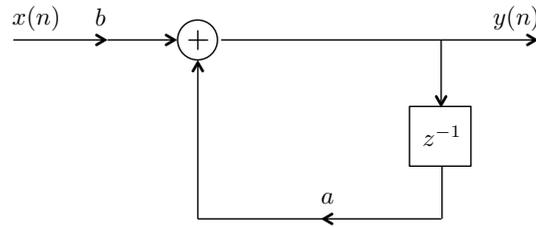
Figure 2: Realisation of a digital filter.
