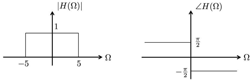
Consider a continuous-time LTI system of which the frequency response is shown above.
